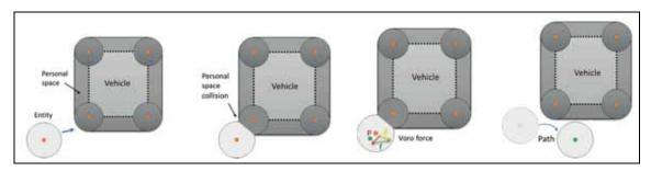
Figure 17. Representation of an entity experiencing a net force f from global path force g and collision penalty force p.
