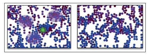
**Figure 11.** North-south bound bidirectional flow. Left: entities disrupting the flow by standing still. Right: an unimpeded corridor captured at the same simulation time as the left scenario.
