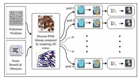
Figure 4. Data-parallel implementation of the CPD method.
